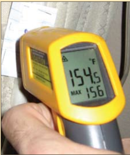
Surface temperature readings were taken periodically using digital infrared thermometers.
